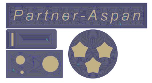
• New command '*Modify* > *Split*': the command can be used to divide a path with the help of one or more blades.
