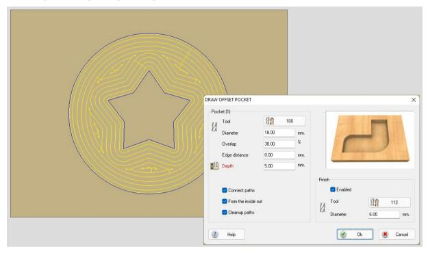
The command allows the **automatic creation of cleaning paths** when an area in which material remains is detected between one offset and the next.
