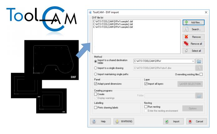
ToolCAM does not create only the coordinate code of an imported profile, but it provides a full CAM environment that allows user to define machining parameters and sequences, to generate an ISO file that is ready for use.
