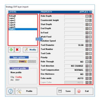
The Advanced DXF import of ToolCAM also allows, through the use of layers and a dedicated processor, to automatically assign machining properties to imported entities:
