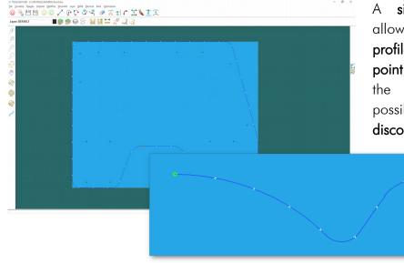
A simplified CAD environment allows you to preview imported profiles, instantly displaying the start point, end point, and direction of the paths obtained. It is thus possible to highlight any points of discontinuity.
